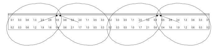
CP-EMW-LED-58 Room Reflectance Avg: 1.03 58 Degree LED Ceiling: Max: 2.96 80 Walls: Min: 0.10 40' Spacing 50 7.5" Mounting Height Floors: Avg/Min: 10.30 20 6' Wide Egress Path Max/Min: 29.60
